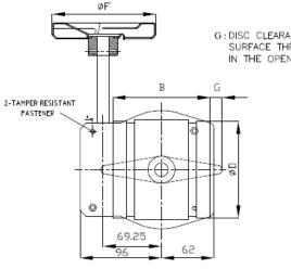
G:DISC CLEARANCE OF BODY SURFACE THROUGH END OF DISC IN THE OPEN POSITION
