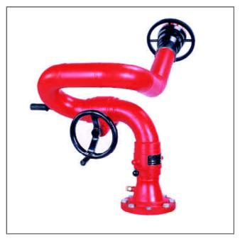
resistant swiveling joint with double row of stainless steel ball bearing. Vertical movement is controlled with handwheel driven enclosed worm gear and twist lock for horizontal movement.
