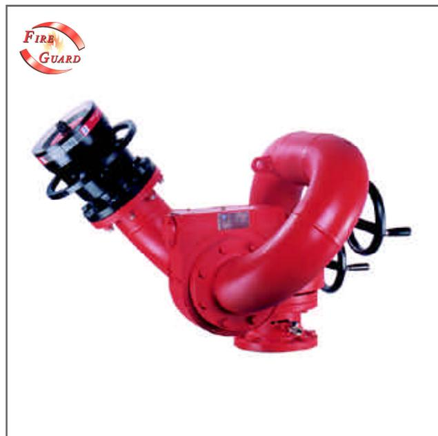
The monitor has large flow capability and can be manually operated by a single fire fighter. The design ensures to prevent jet reaction forces from effecting the horizontal and the vertical position of the monitor. The counter balance is not required to offset the weight of the nozzle. The monitor has the ability for 360 deg. continuous horizontal rotation and angle of elevation is adjustable with fix stop from 90 deg. above horizontal to 65 deg. below horizontal.
