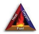
Portable fire extinguishers apply an extinguishing agent that will either cool burning fuel, displace or remove oxygen, or stop the chemical reaction so a fire cannot continue to burn. When the handle of an extinguisher is compressed, it opens an inner canister of high-pressure gas that forces the extinguishing agent from the main cylinder through a siphon tube and out the nozzle. A fire extinguisher works much like a can of hair spray.
