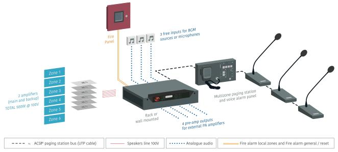
Connection for up to 10 equipment with double communication link. Up to 60 zones and speaker lines.
