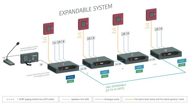
Connection for up to 10 equipment with double communication link. Up to 60 zones and speaker lines. EVAC and ALERT local messages + Autonomous emergency power supply for each ONE unit.
